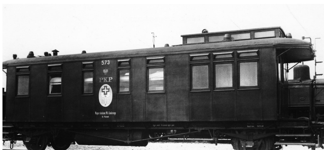
Figure 3. The transport of the wounded at the operational level was to be carried out primarily by rail. Plans for mobilisation included assembling 36 permanent and semi-permanent hospital trains, which could be supplemented by improvised trains. The photograph shows one of the ambulance coaches at Poznań railway station. Source: National Digital Archives
