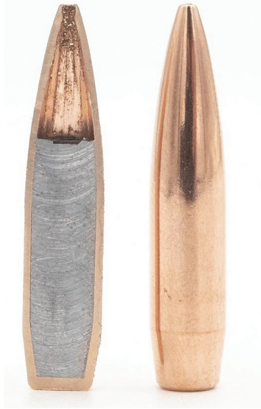
Figure 3. A cross-sectional image of .264, 123 gr. Hollow Point Boat Tail, Lapua Scenar. Source: https://reloaders.eu/lapua-scenar-a-good-hunting-bullet/ [13]
