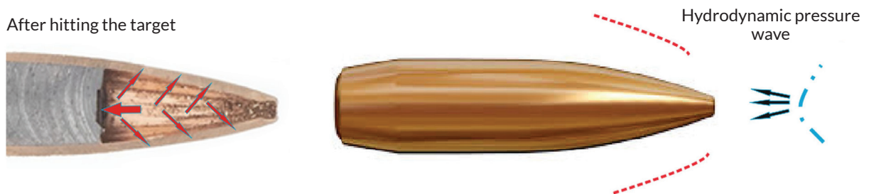
Figure 1. A schematic image of a projectile deforming in a controlled manner (by G. Motrycz)
