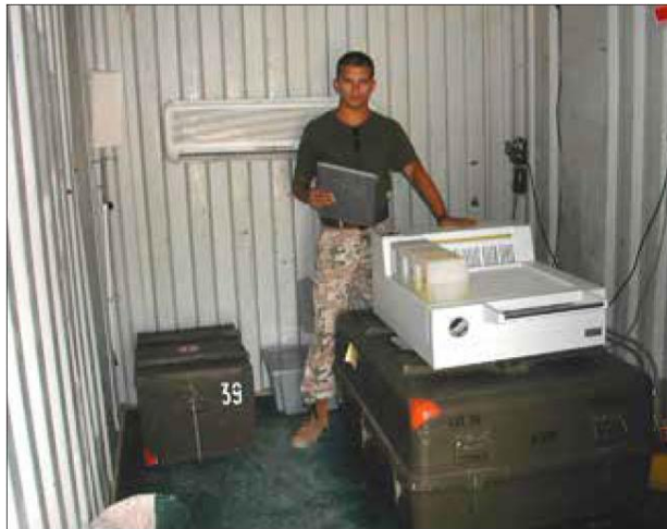
Figure 12. AGFA Curix 69 automatic developer on the transport box in darkroom container. Polish Field Hospital of the Polish Military Contingent in the Stabilization Force in the Republic of Iraq. Camp Lima near Karbala, 2004-2008 (source: authors' collection)
