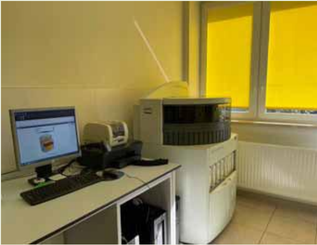
Figure 3. BenchMark ULTRA system - a fully-automated immunohistochemistry and in situ hybridisation system
