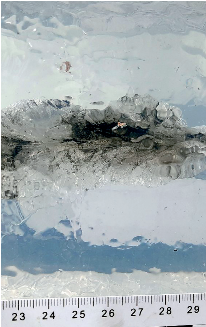
Figure 4. Permanent cavity in ballistic synthetic gelatin created by a .308 Win caliber bullet. Photo by G. Motrycz
